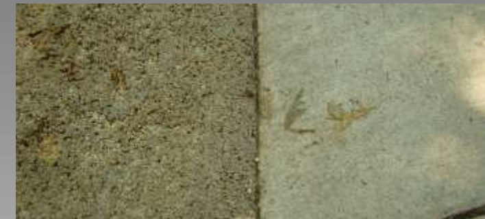
Pervious concrete is shown on the left and regular concrete on the right.
